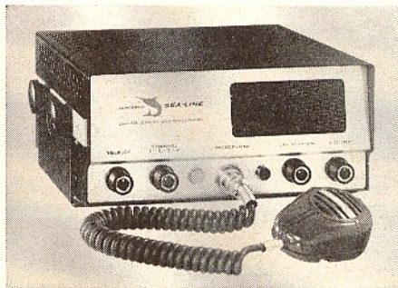
(Left) Canadian Marconi's "Clipper" transceiver is shown mounted on a small boat. (Center) Aerotron "Sea Line," used by commercial and pleasure boaters, has a 35-watt power output. (Right) Dwarfed by its m.f. brothers, this Hammarlund v.h.f. unit is aboard C.G. Cutter "Tamaroa."
