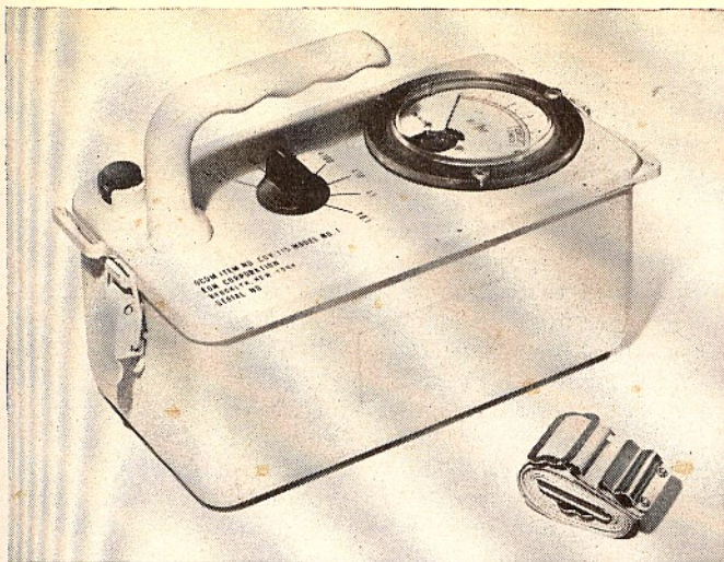
Fig. 4. The CD Model V-715 measures up to 500 roentgens/hour.
